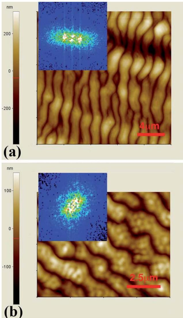
FIG. 3. (a) Topographical grating oriented along the light polarization direction when the linearly polarized beam is focused by means of a spherical lens. (b) The same as for (a) when the light beam is circularly polarized with residual linear polarization along the grating vector. The pictures' insets show the two-dimensional Fourier transform of the topographical maps shown in (a) and (b).
