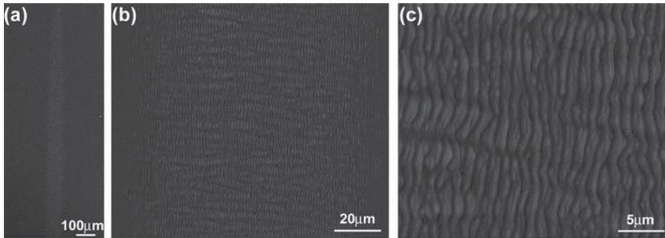
FIG. 1. (a)–(c) SEM micrographs of an elliptical-shaped patterned area, obtained by focusing the laser beam with a cylindrical lens.
