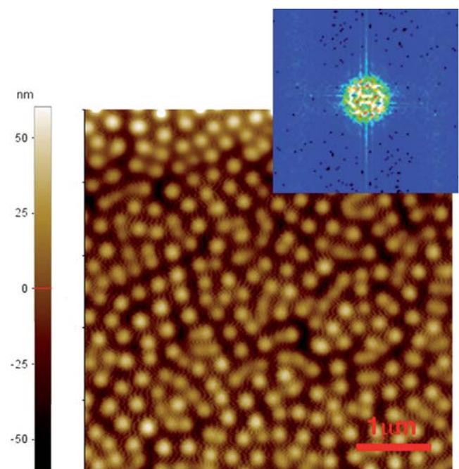
FIG. 4. Spontaneous surface structuring resulting from illumination by means of a 337 nm wavelength laser beam with a low polarization degree. The mean size of each topographical feature (dots) is of about 180 nm.
