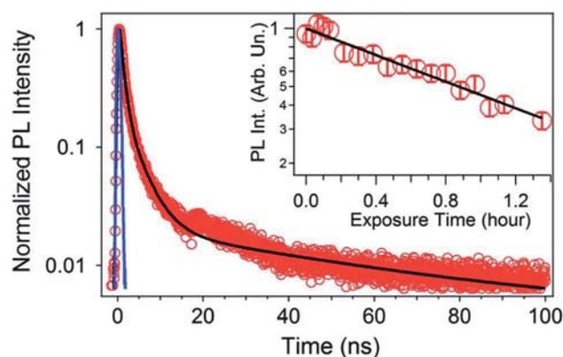
**Fig. 7** Time evolution of the nanocomposite emission. The black continuous line is a fit to the data by the sum of three exponential functions, convoluted with the instrumental response function, displayed as a blue continuous line. Inset: PL decay upon continuous exposure to UV pumping light. The black solid line is a fit to the data by an exponential function.
