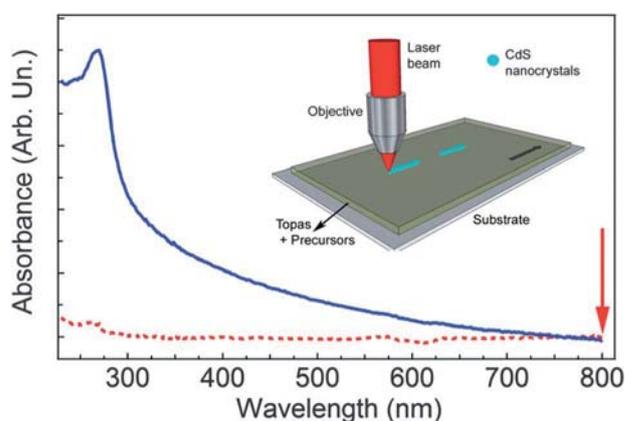
**Fig. 2** Absorption spectra of the TOPAS®-C12 films (continuous line). The absorption of TOPAS® is also shown for comparison (dotted line). The arrow indicates the exposure laser wavelength ( $\lambda = 800 \text{ nm}$ ). Inset: schematics of the laser writing system.
