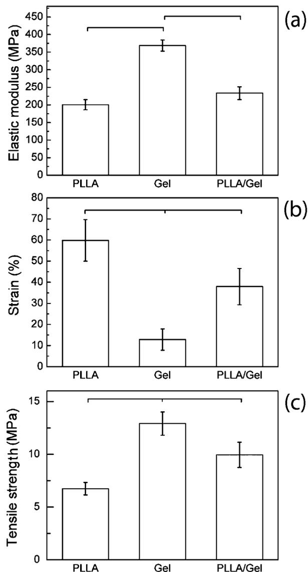
**Fig. 4** Elastic modulus (a), strain (b), and tensile strength (c) of the produced NFs. Results are expressed as (mean  $\pm$  standard deviation). Bars show statistically significant differences ( $P < 0.05$ ).
