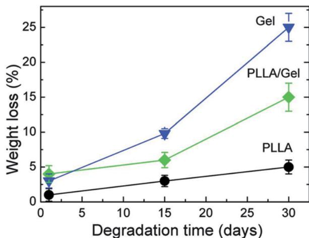
**Fig. 2** Degradation behavior of the electrospun nanofibrous supports, described by percentage weight loss vs. degradation time for PLLA (circles), Gel (triangles) and PLLA/Gel (diamonds) NFs.
