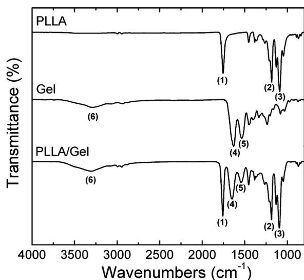
**Fig. 3** FTIR spectra of PLLA, Gel and PLLA/Gel NFs (from top to bottom). Relevant transitions: (1)  $1758\text{ cm}^{-1}$ , (2)  $1185\text{ cm}^{-1}$  and (3)  $1088\text{ cm}^{-1}$  are typical bands of PLLA, whereas (4)  $1629\text{ cm}^{-1}$ , (5)  $1538\text{ cm}^{-1}$  and (6)  $3330\text{--}3600\text{ cm}^{-1}$  relate to the Gel component, respectively.
