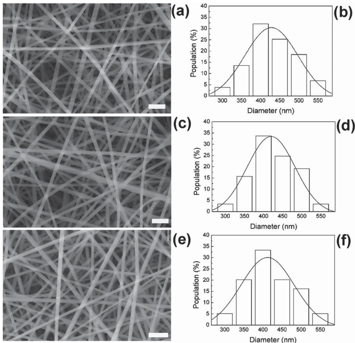
**Fig. 1** SEM micrographs of PLLA (a), Gel (c) and PLLA/Gel (e) nanofibers (scale bar: 2  $\mu\text{m}$ ), and corresponding distributions of fiber diameters for PLLA (b), Gel (d), and PLLA/Gel (f). The superimposed lines are the best fits by Gaussian curves.
