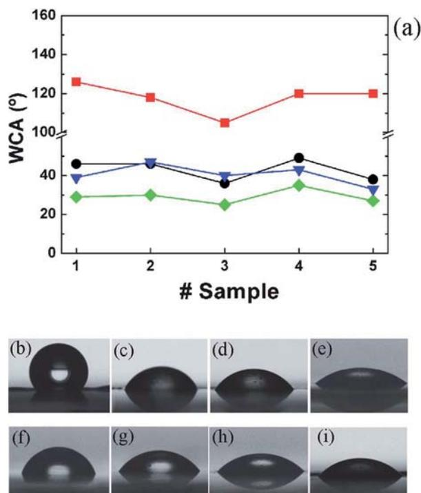
**Fig. 5** (a) WCA values for different nanofibrous scaffolds (# = 1–5) of as-spun (square) and plasma-treated PLLA (circles), Gel (triangles), and PLLA/Gel (diamonds) NFs. Lines are guides for the eyes. Middle panels: optical micrographs of water droplets onto as-spun (b) and plasma treated (c) nanofibrous PLLA (b), Gel (d) and PLLA/Gel (e) surfaces. Bottom panels (f–i) show the corresponding photographs on reference film samples.
