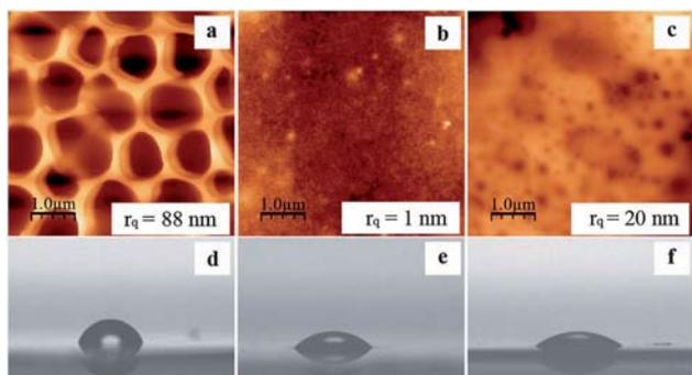
**Fig. 7** Atomic Force Microscopy micrographs of (a) PLLA, (b) Gel and (c) PLLA/Gel (50 : 50) films. Vertical scale bars are 480, 11 and 165 nm, respectively.  $r_q$ : corresponding measured root mean square roughness. Photographs of water drops ( $\approx 2 \mu\text{L}$ ) on the surface of (d) PLLA, (e) Gel and (f) PLLA/Gel (50 : 50) films.
